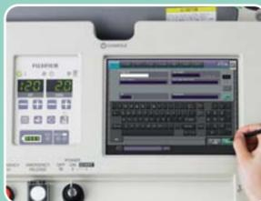
Input patient information with the touch-screen panel. By selecting the exposure menu on the CR Console, exposure factor (kV, mA) will be set on the x-ray operation panel.
