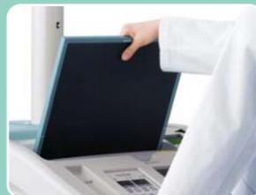
Set the exposed IP cassette. As images can be previewed on the spot, the next processing step can be conducted smoothly. IP cassettes can be used repeatedly and there is no need to carry around numerous cassettes.
