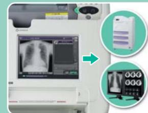
Read images are transmitted to the hospital network from the image processing unit via wireless LAN. Images can also be transferred to the hospital CR Console with USB memory media.
